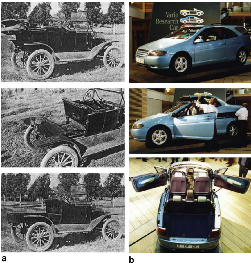
Figure 3 Examples of automotive modularity: then and now. (a) Ford's Touring model (1914): four-seat car to truck (Clymer, 1955), (b) Mercedes' Vario Research Car (2004): wagon to sedan to convertible
