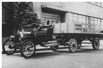
Tractor coupled to semitrailer (Cavette, 2006)
